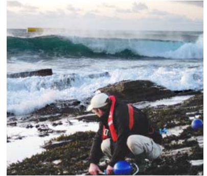
Figure 4. Changing Terobuoy test blocks at Billia Croo (Dwarf algae-Limpet-Barnacle assemblage) - Aquamarine Oyster WEC in background. Source: [1]
