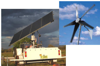
Figure 2: PV powered membrane system and 1 kW FuturEnergy WT.
