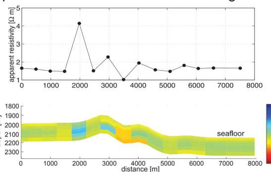
Fig. 3: Resistivity profile and stitched 1D resistivity models can be used to identify highly resistive zones of gas hydrate.
