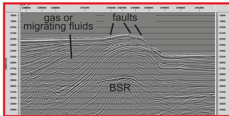
Fig. 1: Depth converted migrated seismic data (05CM-38) clearly resolves a BSR, extensional faulting in the upper layers of an anticline due to tension and wipe-out zones due to migrating fluids.
