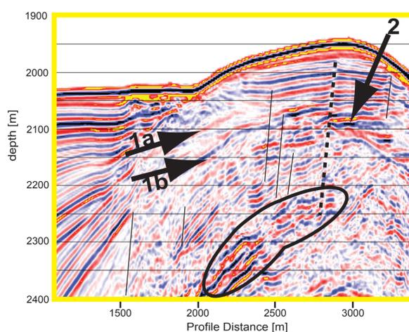
Fig. 2: Resistivity anomalies superimposed on depth converted seismic data with initial interpretation. (See Toulmin et. al. 2008 - AGU poster for more detail)
