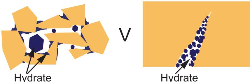
Fig. 4. Hydrate can float in pore space between sediment grains and cement grains together (left), or fill fractures (right). It is unknown how these different modes of hydrate distribution affect apparent resistivity measurements.
