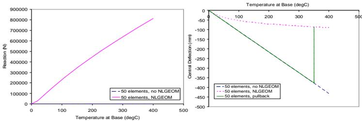
Figure 2: (a) Deflection and (b) reaction in an elastic beam with and without nonlinear geometry when a constant thermal gradient is applied
