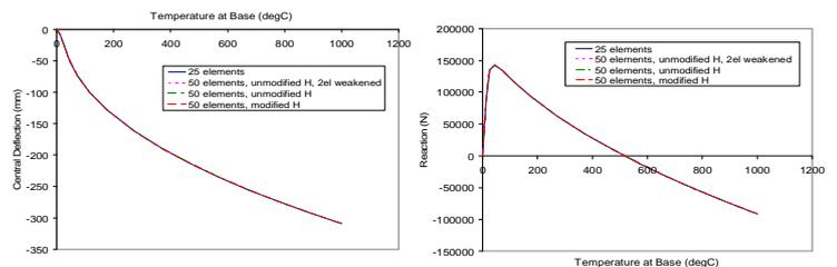
Figure 6: (a) Deflection and (b) reaction in a materially nonlinear beam when both a uniform thermal expansion and a constant temperature gradient are applied with different mesh discretisations and softening modulus.
