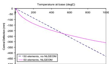
Figure 3: Deflection in an elastic beam with and without nonlinear geometry when a constant temperature increase and a constant thermal gradient is applied
