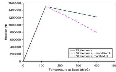
Figure 4: Reaction due to uniform temperature increase in a materially nonlinear beam with different mesh discretisations and softening moduli
