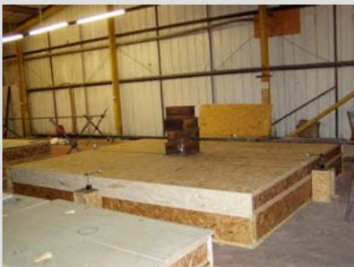
Fig 1a (top row): Test floors during construction
