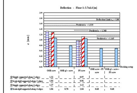
Fig 5: Deflections of a typical floor
