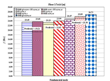
Fig 4: Comparison of predicted & test FNF results
