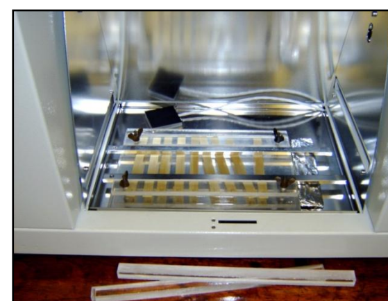
Thin microtomed strips used for colour monitoring and tensile strength tests after being exposed in an Atlas Suntester.
