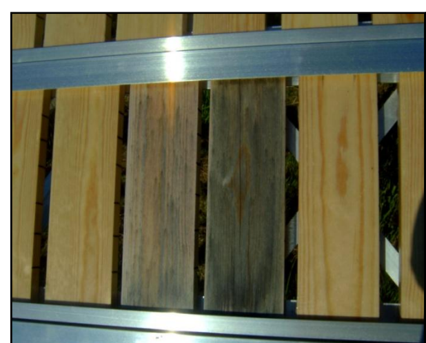
An outdoor exposure experiment showing the differences between coated and uncoated specimens upon natural weathering which includes exposure to solar UV radiation.
