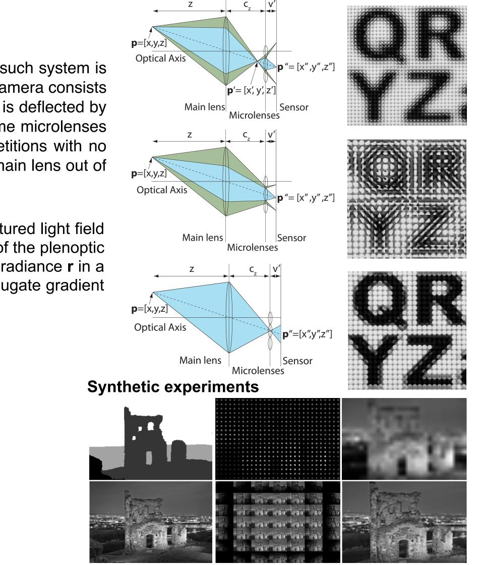
image, **r** is the reflectance, **H** is a sparse matrix representing the point spread function of the plenoptic camera that depends on the depth, and **w** is additive Gaussian noise. We estimate the radiance **r** in a Bayesian framework using the image prior  $\mathbf{p}(\mathbf{r}|\mathbf{a}, \sigma_u) = \mathcal{N}(\mathbf{r}|0, \Sigma_r)$  solved via conjugate gradient least squares.
