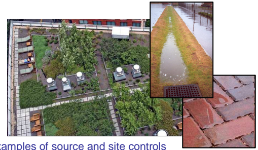
Examples of source and site controls
